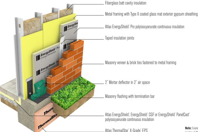
rigid continuous insulation at foundation
